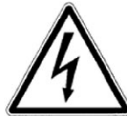
Symbol indicating danger due to electrical power ON.
