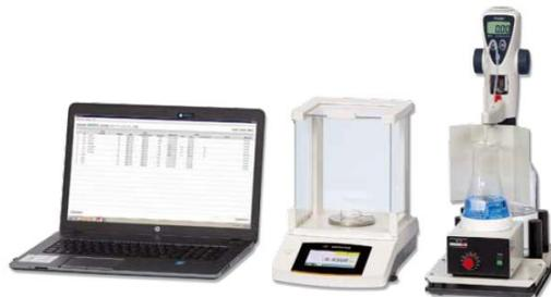
The software receives data from the scales and titration station via USB-interface points, collates and automatically calculates the nitrogen and protein content of the samples. Precise sample classification and manipulation assurance according to GLP are thus guaranteed.
