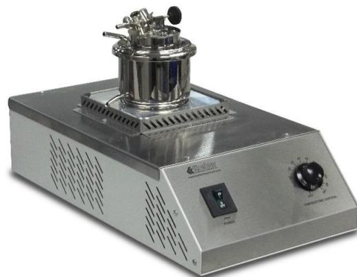
Figure 5: Assembled Tag Closed Cup Flash Point Tester
