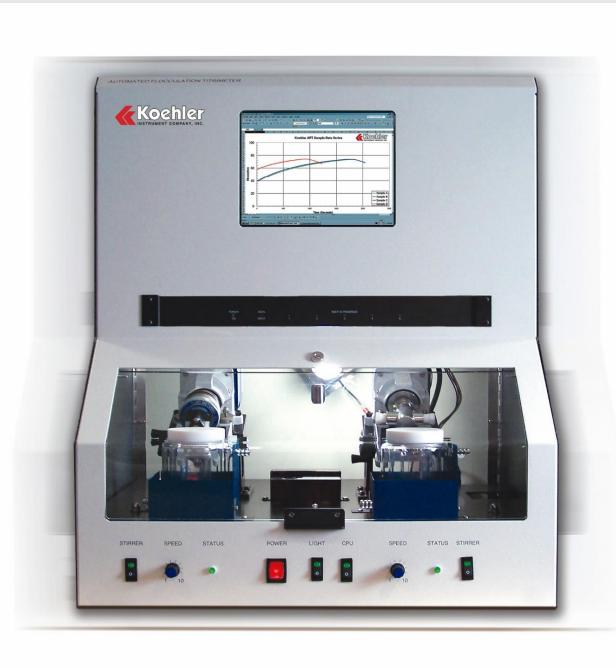
From the FR vs. C plot the X and Y intercepts are measured, where  $FR_{max}$  is the Y-intercept and  $C_{min}$  is the X-intercept. The latter is the ratio of the weight of oil to volume of titrant at the onset of flocculation with zero toluene present.  $FR_{max}$  is the volume fraction of toluene in the toluene/titrant mix at the onset of flocculation at zero oil concentration.
