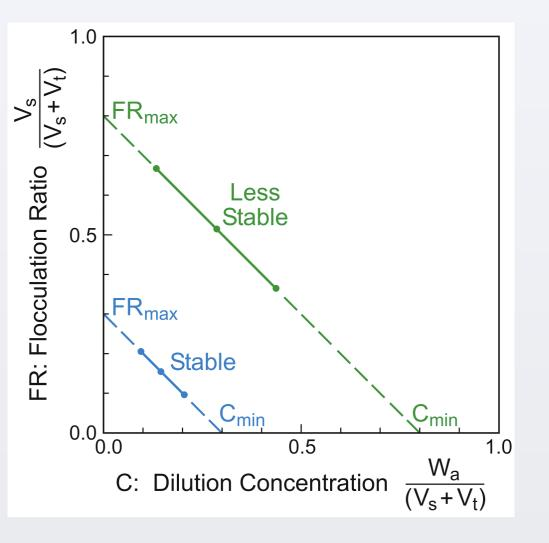
The newly updated Automated Flocculation Titrimeter (AFT) allows users to easily and reliably predict which heavy oils and petroleum residua (including asphalts) can be mixed without causing phase separation or coking. It automates the collection of Heithaus values and predicts flocculation for various crudes.
