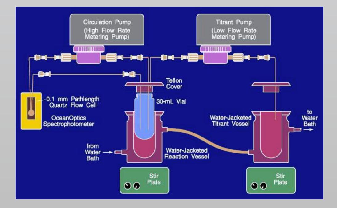
The AFT performs the titration in a closed-looped glass and Teflon system to prevent evaporative solvent losses and to eliminate fouling of metal surfaces, the schematic is shown to the left
