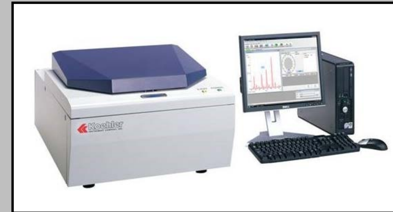
Figure 1: EDX3000 Benchtop EDXRF Elemental Analyzer Description/Features: The following instrument conforms to D7220, and is used for the determination of total sulfur in petroleum, and petroleum products that are single-phase. In the image above the EDX3000 is connected to an external PC computer system, running on the operating system: Microsoft Windows Vista. The EDX3000 can analyze a large array of elements from 11Na to 92U in solids, liquids, alloys, powders, and thin films.
