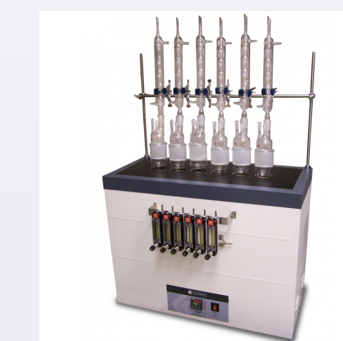
Corrosiveness and Oxidation stability Test Apparatus
