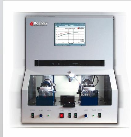
The Automated Flocculation Titrimeter (AFT) pictured to the left was developed to perform ASTM D6703 which measures the state of the dispersed particle system and calculates predictive parameters for heavy oils.
