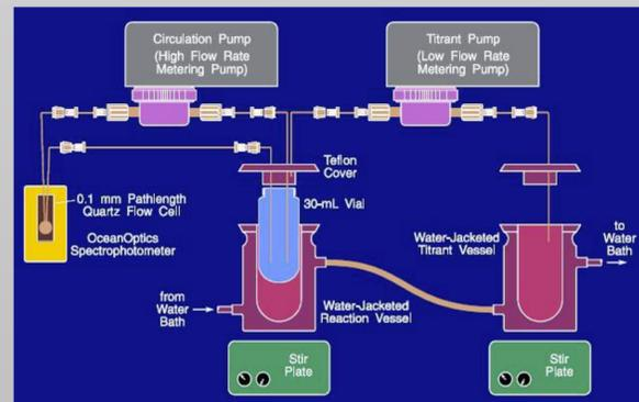
The AFT performs the titration in a closed-looped glass and Teflon system to prevent evaporative solvent losses and to eliminate fouling of metal surfaces, the schematic is shown to the left
