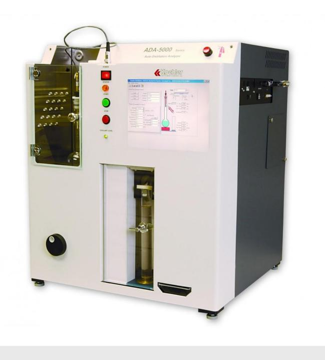
Recent discussion for changes to ASTM D86 involve safe and logistical concerns. The currently used Mercury thermometer is undergoing a possible change to a Gallium thermometer and the chilling requirement for Group 1 fuels may be removed.
