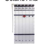
Figure 10. K41506 Fluorescent Indicator Adsorption Apparatus
