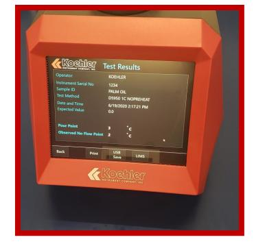
After the test ends, a result screen will display all the data and there will be an option to print and save the data.
