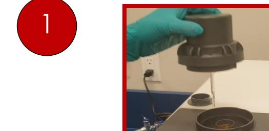
Select the appropriate head for either Cloud or Pour Point testing. The instrument will automatically detect which head has been selected.
