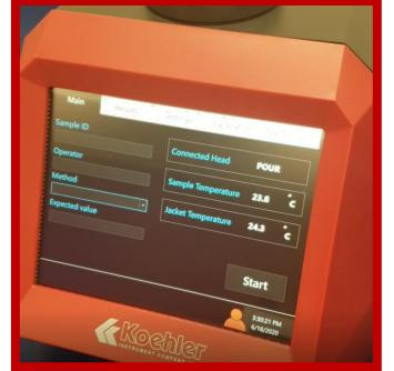
The instrument will prompt the user to enter the sample ID, operator, and select a test method before the test can begin.
