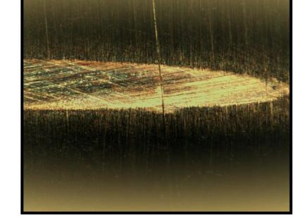
For good friction behavior, the edges of the wear scar taper off.
