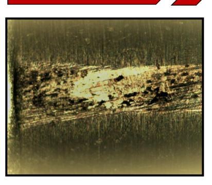
For bad friction behavior, the cylinder roller tilts due to adhesive events, resulting in a widened wear scar.
