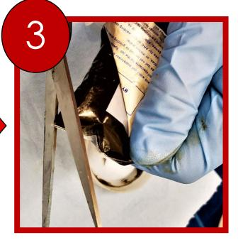
Cut the tip off the bag and use this opening to fill a syringe to at least 5 mL, occasionally tapping the syringe on the lab bench to pack the grease tighter. Make sure there are as few air pockets as possible.
