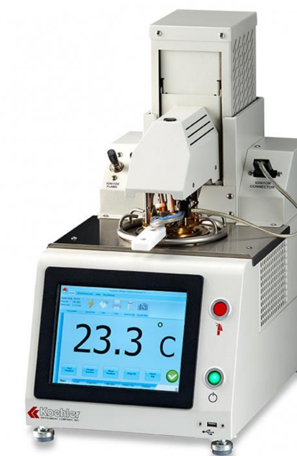
Figure 1. The Automatic Pensky-Martens Closed Cup Tester shown with the startup display, and a closed hood ready for testing flash points.
