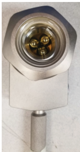
Figure 2. A typical four ball test setup before test specimen is placed in the cavity
