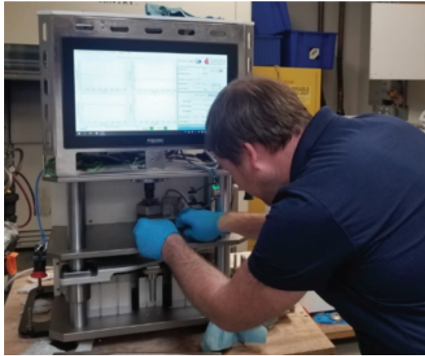
Figure 3. The Koehler Benchtop Four Ball Tester during the manufacturing stage
