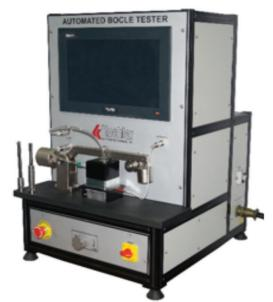
Figure 3: Image of the K94190 Lubricity Test Rig (BOCLE) by Koehler Instrument Co.
