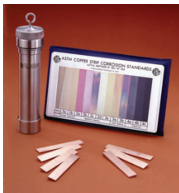
Figure 2. Copper Strip Corrosion Test Bomb Bath
