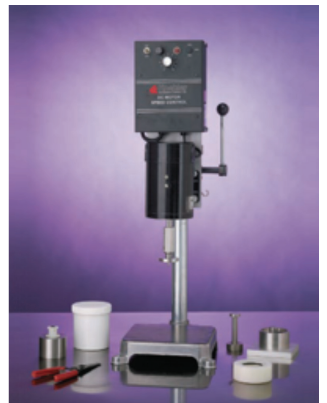
Figure 3. Rust Preventative Properties of Grease Instrument
