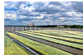
Figure 4. The image to the right is of Algae System's half-acre algae photobioreactor located in Daphne, Alabama, where algae is harvested in floating mobile pods for biofuel production, and is connected to the city's wastewater treatment system.
