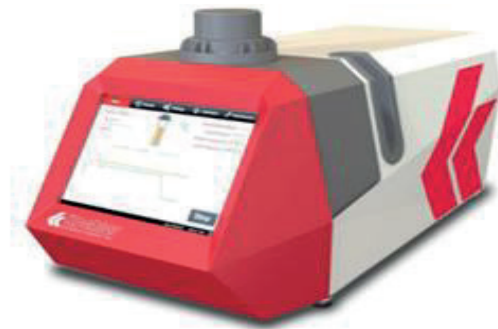
Figure 1. K77000 Automatic Cloud and Pour Point Analyzer
