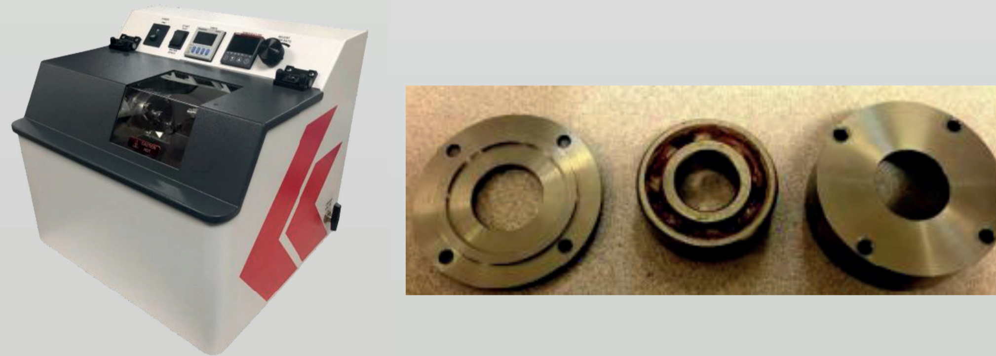
Figure 3. Koehler's Water Washout Tester (left) and bearing housing for grease to be tested (right).
