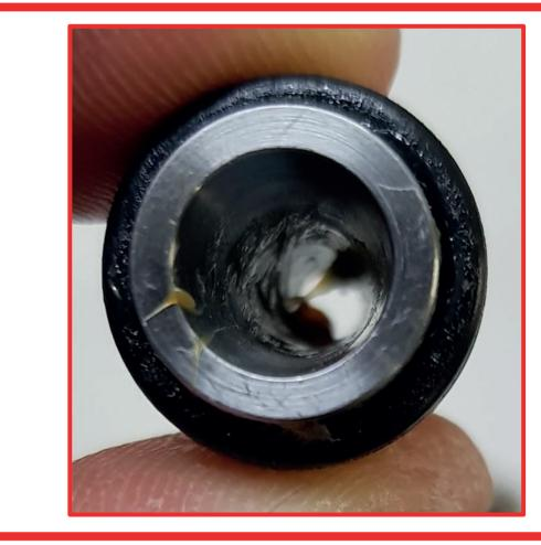
intervals, pressurizing one side of the nozzle. At a certain pressure the grease will squeeze out of the nozzle. The instrument will take note of that pressure and displayed it on the screen of the K95300, concluding the test.
