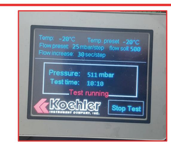
4. Once the grease has been squeezed out, there will be a pressure drop and the machine will display the pressure and offer to end the test or save the results to a USB flash drive:
