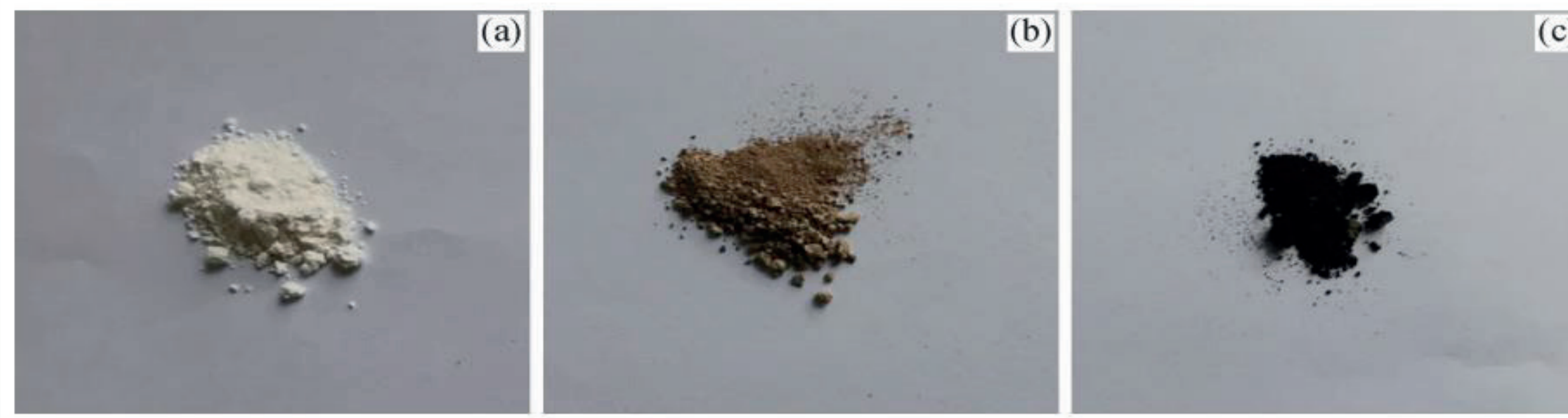
Oxidation of Lithium 12-hydroxystearate soap after (a) 0 hours (b) 36 hours (c) 72 hours
