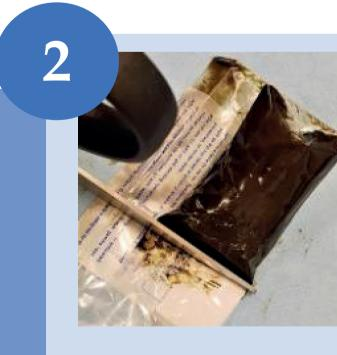
Pack the grease sample into a small plastic bag, using a flat-edged tool to push the sample into an area as tight as possible at the corner of the bag to minimize air pockets.
