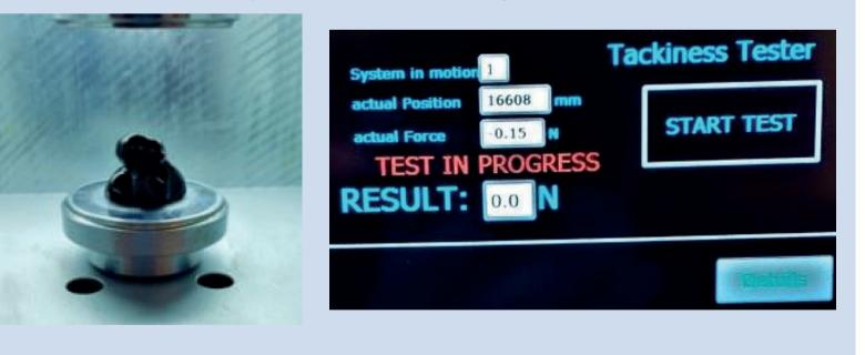
Wait for the instrument to complete testing. Measurements of the tackiness of the grease sample will be displayed on the data screen of the instrument.
