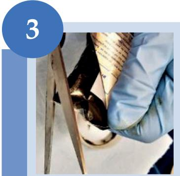
By snipping the tip of the bag, fill a syringe with at least 5 mL of the grease sample. Be sure to remove air pockets by tapping the syringe against a lab bench while filling the syringe.
