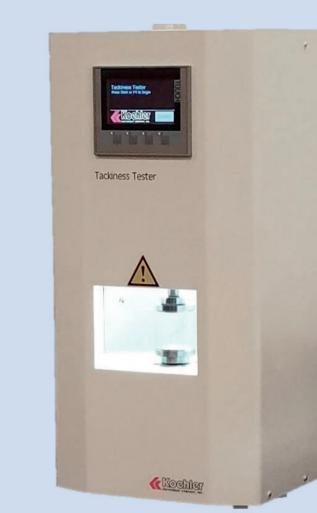
reproduced consistently. By eliminating the subjectivity of the finger test, the K95200 allows for grease tackiness to be accurately compared between different testing personnel.
