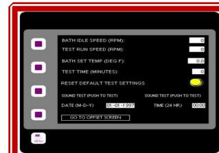
Prior to running a test, check all the testing setting. The default setting is for ASTM D7548 method or use custom parameters.
