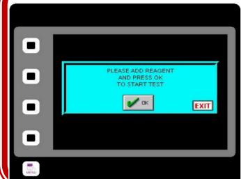
After pour 50 mL of sample into the test jar and start the test, the sample will be stirred at 900 RPM for 1 hour under default.
