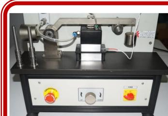
The parts of the K94190 instrument should be assemble according to the instructions on the operation manual. 50 mL of fuel is added into the fuel bath.
