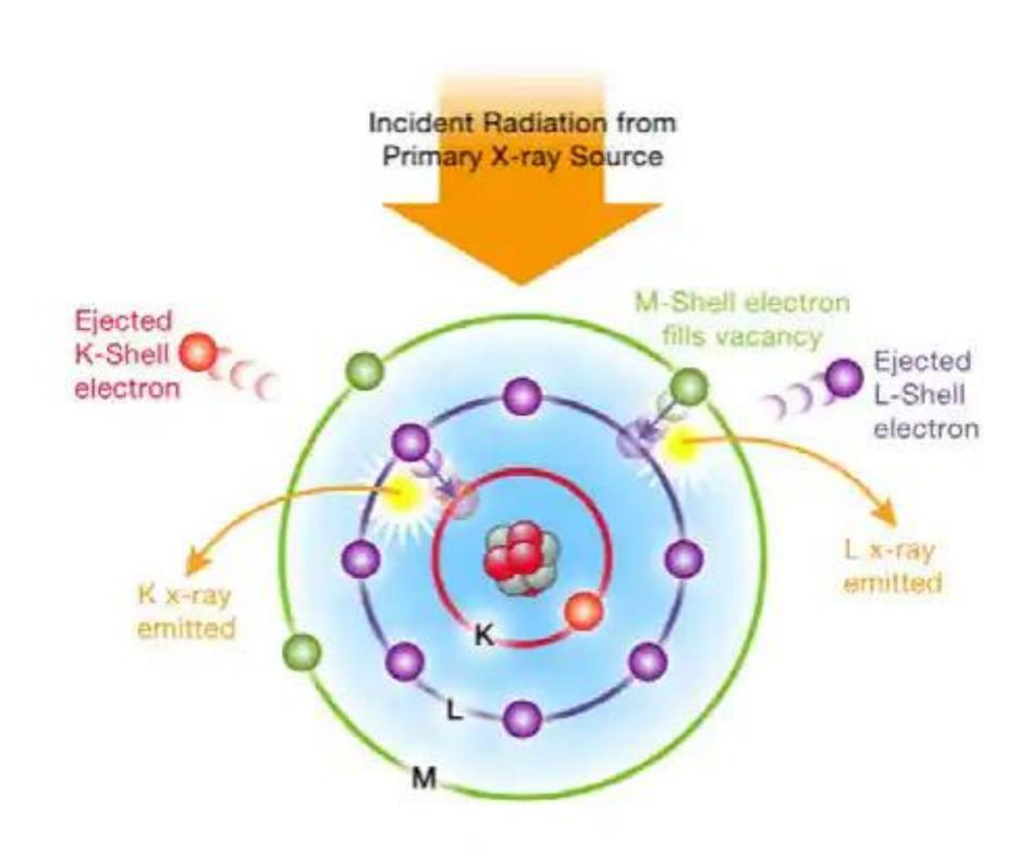
The fluorescent x-rays have "peaks" visible on a light spectrum. The location of a peak will indicate which element is present, and the size of the peak will indicate concentration of the element in the mixture
