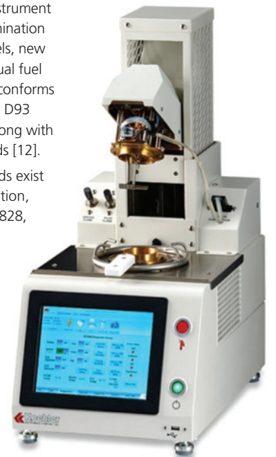
Figure 2: The K71000 Automatic Pensky-Martens Closed Cup Flash Point Tester, capable of measuring flash point as per ASTM D93 [11]
