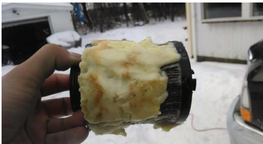
Figure 3: The formation of solid wax crystals from diesel use at cold temperatures, leading to the plugging of the fuel filter [19]
